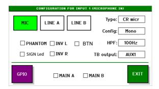
The "overload" LED next to each input fader marked "O" is a dual color version, this will light red in case of an overload. The check box 'SIGN Led' activates the "Input signal present". The led will turn green if there is a signal of at least – 25dB present at the input.
