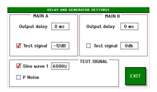
You can insert a delay in each of the stereo outputs channels for up to a maximum of 100 msec. This delay can be used to compensate for the latency in video processing systems to maintain synchronization of picture and audio. Another application is the delay of (a group of) loudspeakers in small PA systems.
