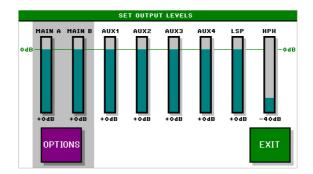
Selecting the OPTIONS button in the output levels screen opens the settings for delay and tone generator.
